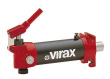
Mechanical safety ensured by an end-of-travel stop and high pressure seals at the back of the piston, which remain effective even in the event of impact on the piston. Automatic piston return. Virax rams are individually tested and inspected.
