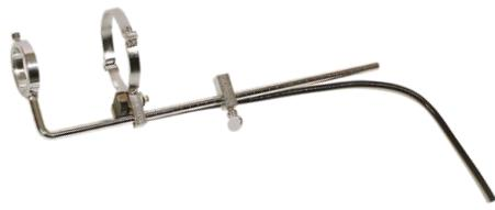
This mechanism enables the same bends to be reproduced on the electric motor hydraulic benders with cylinder No.2 (240802).
