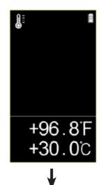
To start a new measurement, press and hold the "Temperature measurement" selection switch again.
