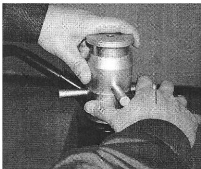
Step 7: Once locked ensure that the distance between the set nut and the hydraulic cylinder is 2.11 mm.
