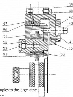
The large upper roller couples to the large lathe screw at a distance of 19mm.
