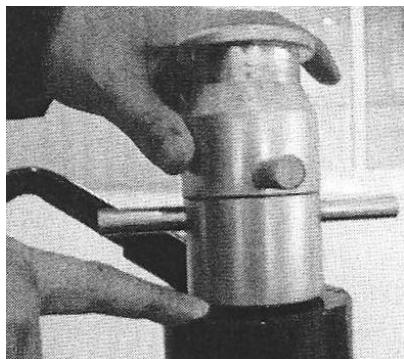
Step 8: Start the machine, pull back the upper roller as far as possible, close the cylinder cutoff valve and start to pump. Do not pump continuously, allow the tube to rotate three times for each pumping operation. When the set nut touches the hydraulic cylinder stop pumping and do not stop the machine until the tube has rotated three times. Stop the machine, open the cylinder cutoff valve to ensure that the hydraulic cylinder recedes and remove the tube.
