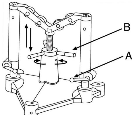
Loosen the lathe screw levers (A) by turning anticlockwise. Take the lathe screw wheel (B), turn it and adjust the tube to the knurling measurement.
