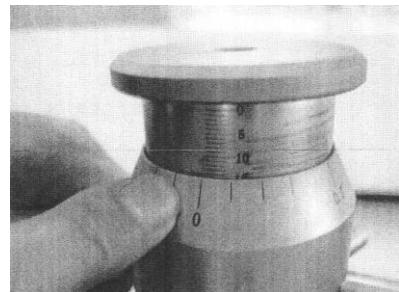
Step 5: Fix the groove depth. For example for 4" the depth is 2.11mm. Pull back the jamb nut 2.11mm on the vertical scale. Each line of the circular scale is equivalent to 0.1mm.
