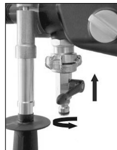
Water pump connection mechanism
