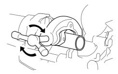
• Turn the tube cutter wheel evenly to the right until the end of the cutting operation. (The wheel must be turned about a quarter of a turn per revolution of the tube).
