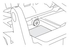
**Important:** Never cut a thread on a tube without a sufficient oil flow. You risk damaging the tube, the die and the machine.
