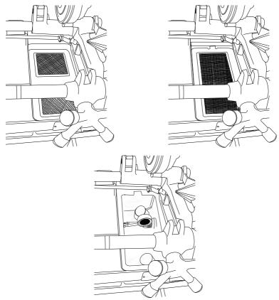
Note: The strainer can also be removed to facilitate cleaning.
