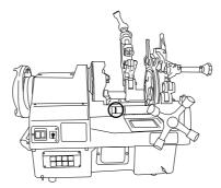
The saddle must not go past this limit: doing this will tear the thread and could even cause the tube to crack.
