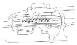
Note: The 1/4 G and 3/8 G markers refer to the BSPT thread standard (G for Gas). The other markers refer to the BSW standard.
