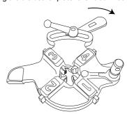
Unscrew the die bearer plate tightening lever and move the plate to the left as far as the stop:
