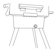
Note: Drain the machine also when it is being transported over any significant distance.
