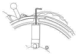
Use the key to remove the jaw retaining screw.
