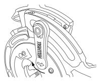
Holding the setting lever, position the scale such that the indication "Remove dies" is opposite
