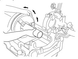
To loosen the chuck, give successive blows in the opposite direction.
