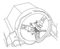
The front chuck jaws must be replaced when they show signs of wear. (Set of 3 jaws for the 162120: part no. 753069)
