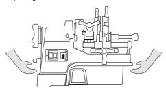
**Warning:** Two people are needed to raise the machine. Raise and move the machine only by using its handles. (The other parts of the machine do not give a secure grip).
