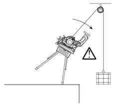
The machine is not intended for coating the threads with sealing paste.
