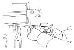
Put the new reamer in place and reposition the gudgeon.
