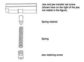
Important: Be careful not to lose the jaw transfer set screw inserted in the side of the jaw.
