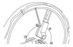
Dismantle the jaw holding plate - crown assembly (or ask a colleague to hold the crown by the spindle nose while you remove the jaw holder):
