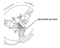
• Replace the spring retainer, spring and screw and tighten the jaw fastening screw.
