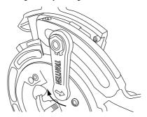
Note: The word "Tighten" is written on the lever accompanied by an arrow pointing anticlockwise. This arrow indicates the tightening direction.
