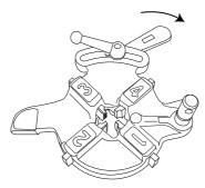
• Position the die bearer plate according to the tube diameter and the desired external thread diameter (see page 29); tighten up the lever.
