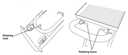
Place the machine on its support, rear of the machine towards the handle, and fix the retaining screws provided with the trolley.
