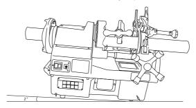
This slope prevents oil flowing towards the back in the tube. Check therefore that this slope is maintained where work is to be carried out.
