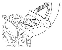
Warning: Do not forget to tighten the gudgeon after replacing the wheel.
