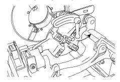
Position the scale to bring the indication corresponding to the tube diameter up to the marker:
