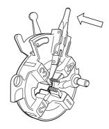
Loosen the cam bearer plate locking lever by turning it in the reverse direction to that indicated by the arrow:
