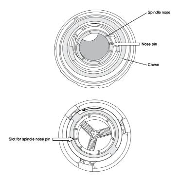
• Screw the jaw holding plate back onto the spindle nose.
