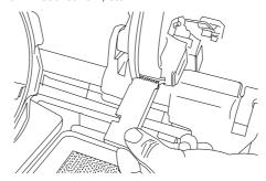
Insert each die until you can feel that the die is blocked by the ball inside the socket.
