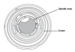
Put the jaw holding plate down, rear facing upwards, and unscrew the jaw holder helical drive ring:
