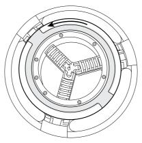
• Turn the jaw holding plate over and remove the three jaw holders:
