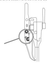
Position the required line opposite the marker (the leftmost line gives the greatest thread length and the rightmost line gives the shortest thread length).
