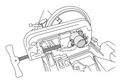
• Turn the tube cutter wheel evenly to the right until the end of the cutting operation. (The wheel must be turned about a quarter of a turn per revolution of the tube).
