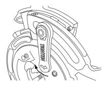
Note: The word "Tighten" is written on the lever accompanied by an arrow pointing anticlockwise. This arrow indicates the tightening direction.
