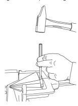
• Remove the cone, replace it with a new one and replace the gudgeon.
