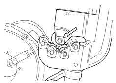
Warning: Do not forget to tighten the gudgeon after replacing the wheel.
