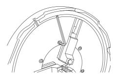
• Dismantle the jaw holding plate - crown assembly (or ask a colleague to hold the crown by the spindle nose while you remove the jaw holder).
