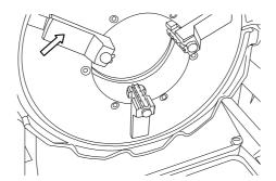
The jaw holders must be replaced when they show signs of wear. (Jaw holder for the 162140: part no. 753070)
