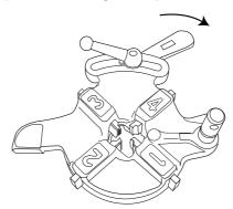
• Position the die bearer plate according to the tube diameter and the desired external thread diameter (see page 32); tighten up the lever.
