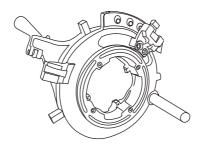
The 4" die head is for cutting threads in 2  $\frac{1}{2}$ " to 4" tubes. The two thread standards which can be used with this head are BSPT and NPT. (One 4" head is dedicated to each of these two standards).
