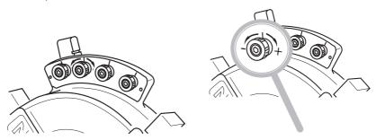
Note: The setting thumbwheels have marks allowing the thread outside diameter to be set finely:
