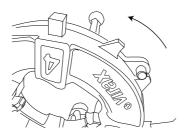
• Go to the side opposite the operator, disengage the notch pointer and, holding the pointer support, tilt the die bearer plate down to its stop:
