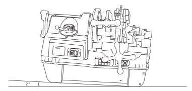
This slope prevents oil flowing towards the back in the tube. Check therefore that this slope is maintained where work is to be carried out.
