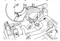
Position the scale to bring the indication corresponding to the tube diameter up to the marker:
