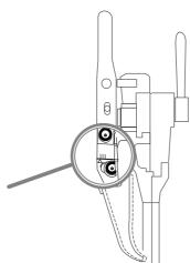
• Position the required line opposite the marker (the leftmost line gives the greatest thread length and the rightmost line gives the shortest thread length).
