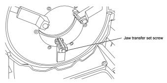
Replace the spring retainer, spring and screw and tighten the jaw fastening screw.
