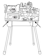
**Warning:** Four people are needed to raise the machine. Raise and move the machine only by using its handles. (The other parts of the machine do not give a secure grip).
