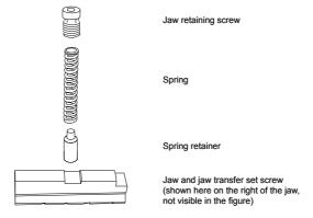
Important: Be careful not to lose the jaw transfer set screw inserted in the side of the jaw.
