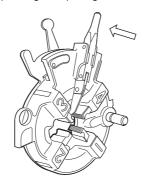
Loosen the cam bearer plate locking lever by turning it in the reverse direction to that indicated by the arrow:
