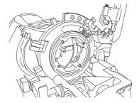
Pull the head housing unlocking handle (marked "Open") and tilt the head to lock it in its housing.
