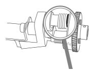
Note: The dies open when the cam roller reaches the end of the cam and drops.
