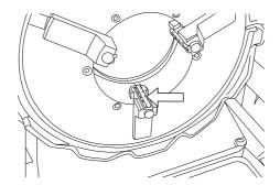
The front chuck jaws must be replaced when they show signs of wear. (Set of jaws for the 162140: part no. 753071)
