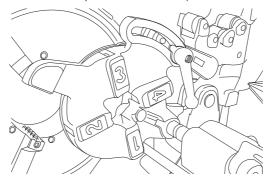
• Tilt the head to mount it in the die head support block (see above).
