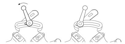
Remove the anti-stop finger from its socket and move the plate to the left up to the stop, which frees the dies.
