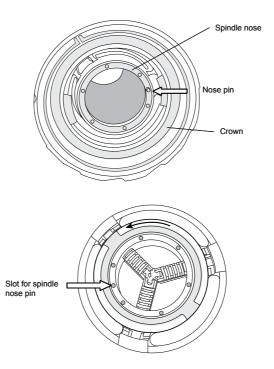
• Screw the jaw holding plate back onto the spindle nose.
