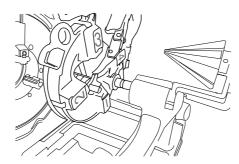
• Tilt the head to lock it in the die head support block (see above).
