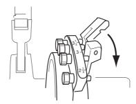
Position the scale so that the indication corresponding to the tube diameter is opposite the lever.
