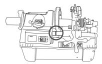
The saddle must not go past this limit: doing this will tear the thread and could even cause the tube to crack.
