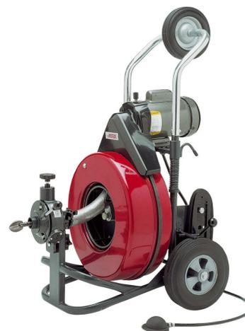
Ø 16 mm (also exists in Ø 19 mm) 30 m long cable (extendible to 60 m) composed of a robust steel wire rolled around a 49-strand thermally treated metal core.
