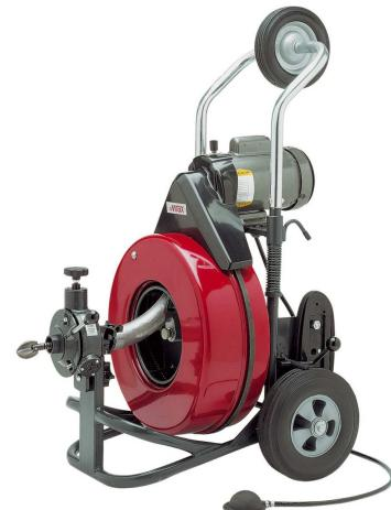
Ø 16 mm (also exists in Ø 19 mm) 30 m long cable (extendible to 60 m) composed of a robust steel wire rolled around a 49-strand thermally treated metal core.
