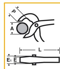
Instant opening by secured locking push-button of the adjusted position by quadruple rack. Ratchet-like operation for fast screwing / unscrewing.
